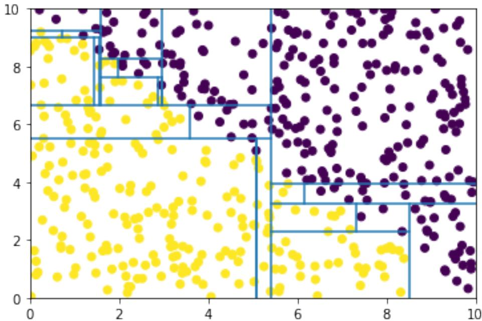
Here, we can see exactly what we were expecting: not being able to use an oblique line, the decision tree creates rectangular areas that are smaller and smaller as the tree grows. Note how each of the final rectangles represents a leaf in the decision tree. We are using a default configuration for the decision tree: this configuration grows until all leaves are pure: indeed, you will see that there are no rectangles containing nodes from both classes.
