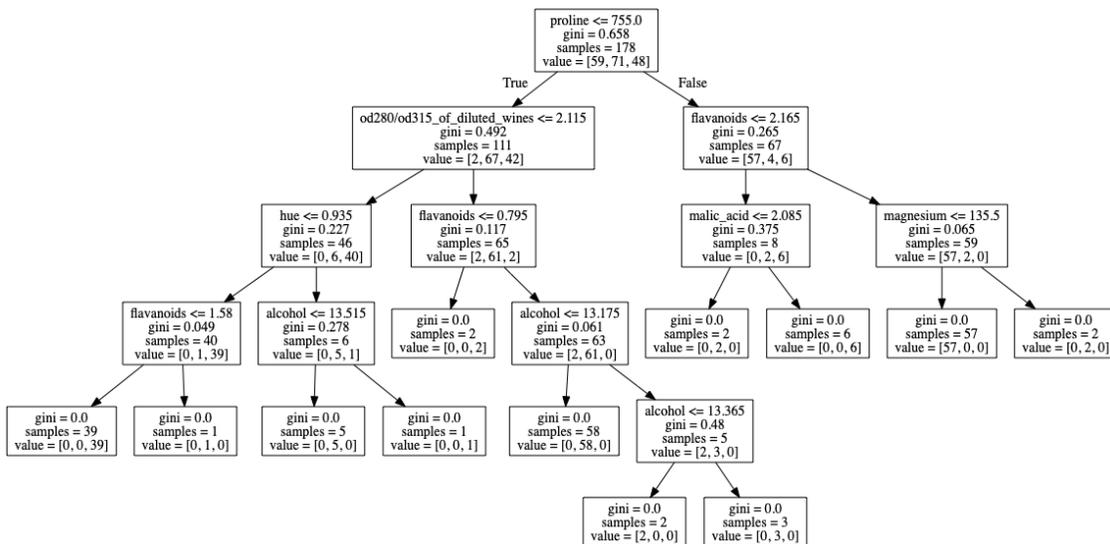
For, notice how each split generates two branches: as can be seen from the root split, the convention used is that the left-most branch is the one selected when the comparison yields a “true” value, the right-most one if the comparison is false.
