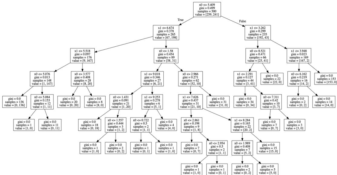
As expected, the decision tree is not capable of separating this linearly separable problem with a “simple” solution. We can say that the tree is not “learning” the underlying rationale behind the data. Instead, it tries to approximate the data as best it can with what it can do.
